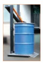
We often collaborate with our customers to develop industry specific lifts. Based on the LoadLift 500, this version has been adapted to handle oil and cable drums.
