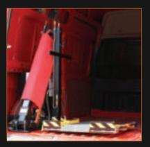
The York adaptation LoadLift as used by Royal Mail is a lightweight and compact lifting platform for loading containerised goods via the rear doors. It is especially useful for handling roll cages and similar items that can be rolled on and off its platform.
