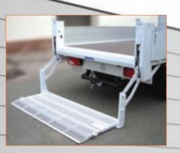
With the same 500kg capacity as our aluminium AP models, the EL500MP comes with an innovative mesh platform. This reduces the weight of the lift, increases vehicle payload and improves fuel consumption. Alternatively, the SP steel platform model can be specified. The standard platform size is 600mm with an additional 200mm toe.
