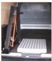
LoadLift 500 is the 500kg capacity rear access platform lift. Platform sizes can be increased to suit the vehicle's rear opening.
